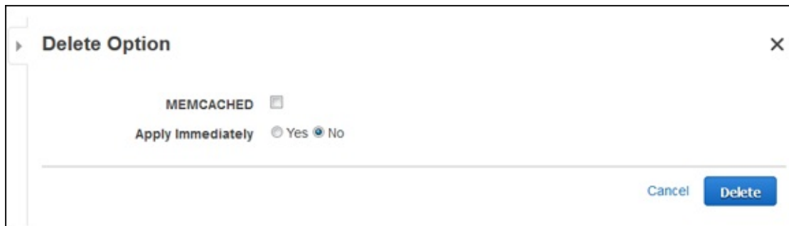
FIGURE 12-8: Use the Delete Option page to remove options from the option group.
